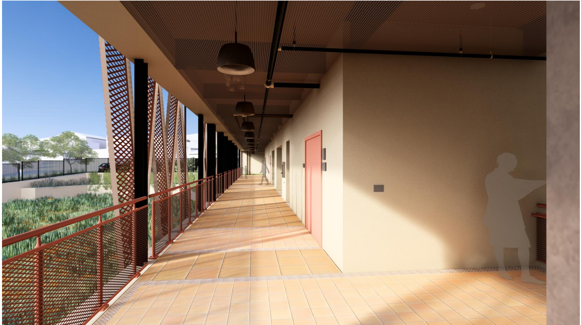
2 nd Floor Covered Breezeway W/ Expanded Metal Mesh Panels
